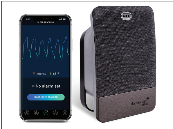
FIGURE 1. SleepScore Max app, a validated noncontact at-home monitoring system designed to measure the user’s sleep.
